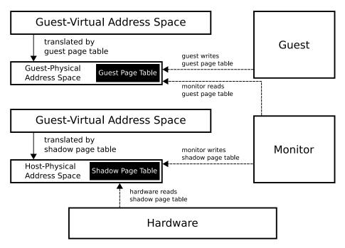
Figure 2.3: The shadow paging mechanism. The monitor reads the page table the guest has written and translates all the entries into a shadow page table. The hardware will then use this shadow page table to perform the actual address translation.
