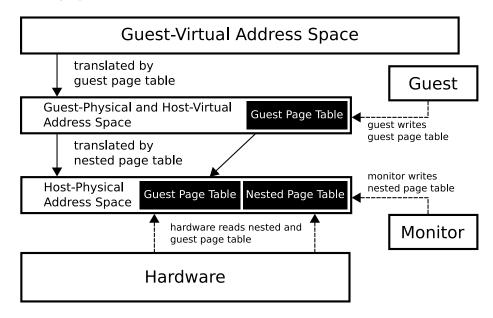
Figure 2.4: The nested paging mechanism. The hardware translates guestvirtual addresses first using the the guest page table and the resulting guestphysical address using the nested page table. The guest page table resides in guest-physical memory which is virtual to the host and therefore all accesses to the guest page table need first to be resolved by the nested page table.
