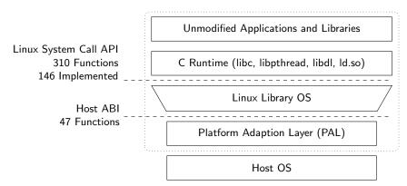
Figure 3.1: Graphene architecture overview.
