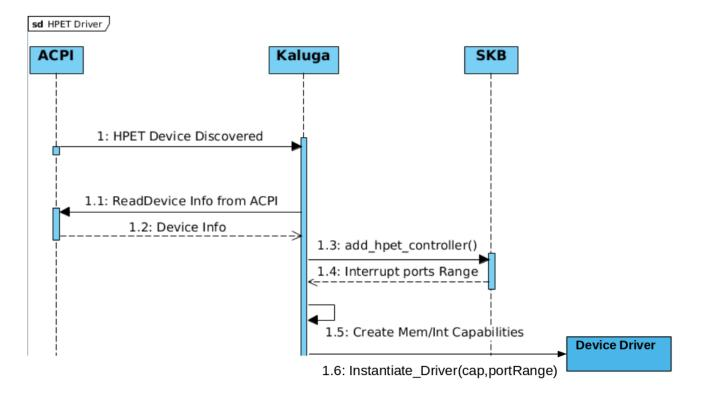
Fig4. Sequence Diagram of Driver Instantiation
