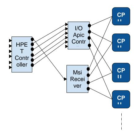
Fig3. Interrupt Model applied on the HPET Controller
