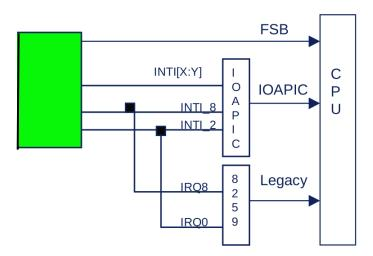
Fig2. HPET interrupt mapping
