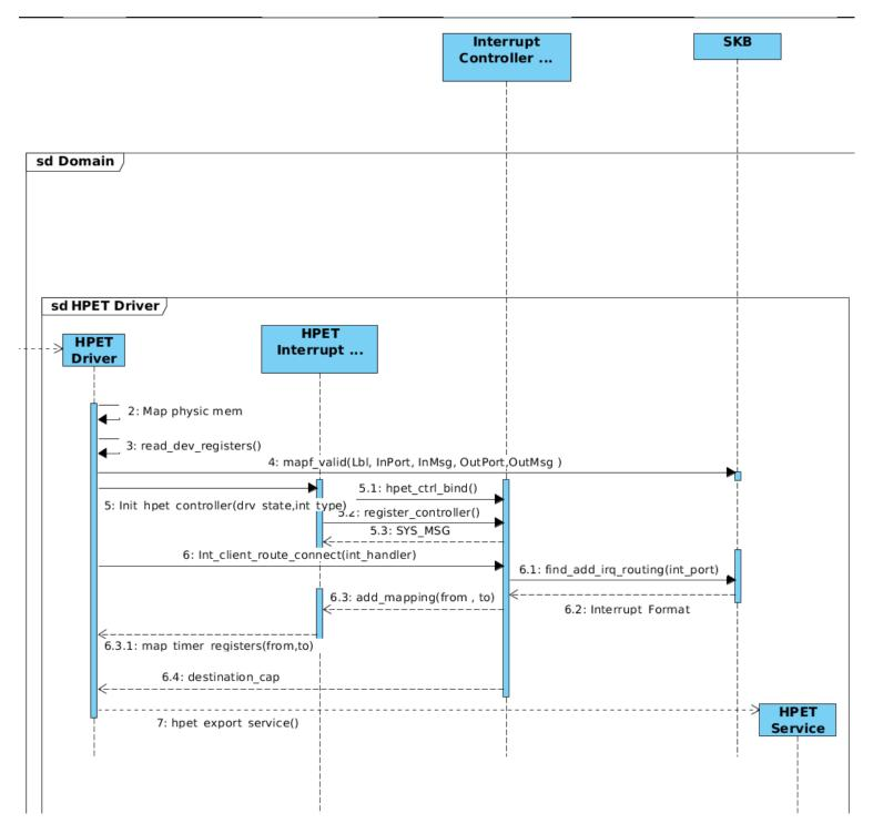
Fig5. Sequence Diagram of the driver's workflow
