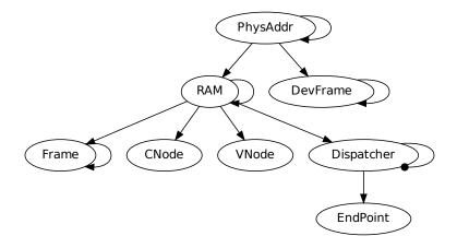
Figure 1: Barrelfish's capability inheritance tree. Taken from [TN013]
