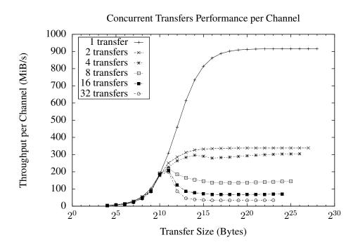
Figure 11: Throughput per channel when simultaneously running up to 32 transfers in parallel.
