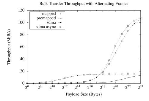
Figure 18: Throughput of bulk transfers using different payload sizes. The memory region used in the request was alternated between eight different frames.
