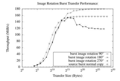
Figure 10: Performance of image rotation by using the double-index addressing mode on the destination with burst mode enabled for both source and destination, compared to a normal copy transfer with burst mode on the source port only.
