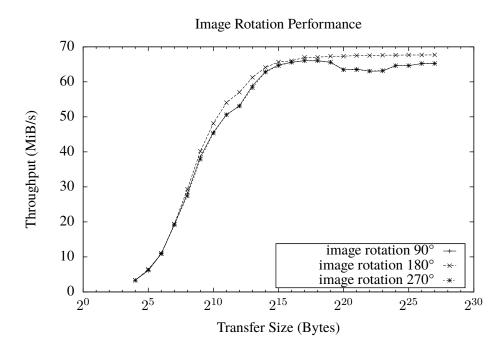
Figure 9: Performance of image rotation by using the double-index addressing mode on the destination. Element and frame size was chosen to represent a nearly quadratic image.
