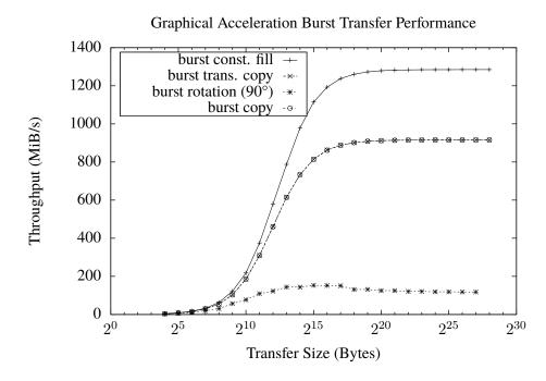
Figure 7: Performance evaluation of using burst transfer mode for the graphical acceleration features such as constant fill, transparent copy and image rotation, compared to normal burst copy. Note that there is no performance difference between normal copy and transparent copy in burst mode.
