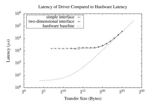
Figure 13: The latency of the two interfaces for different transfer sizes compared to the latency of the direct use of the device.
