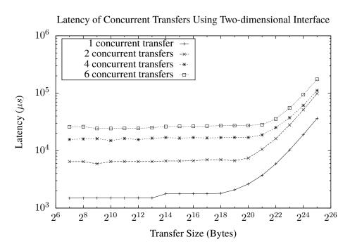
Figure 15: Latency per client when issuing concurrent transfers. The duration of individual transfer increases with the number of concurrent transfers
