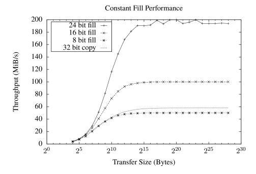
Figure 5: Performance of the constant fill graphical acceleration feature, using color values of size 8, 16 and 24 bits. The spikes when using a 24 bit fill value where consistent in all measurements.
