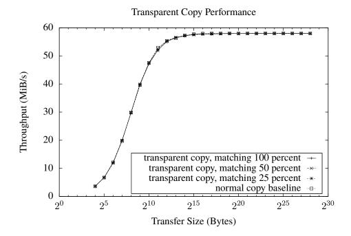
Figure 6: Performance of the transparent copy graphical acceleration feature, using an element size of 32 bits with a 24 bit comparison value. Note that the percentage of matching elements has virtually no impact on performance.
