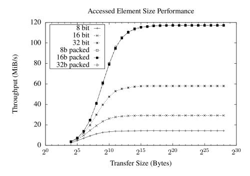
Figure 3: Impact of the element size (8, 16 or 32 bits) on the throughput for different transfer sizes. It can be seen that since the optimal amount of elements are transferred in packed access, the chosen element size becomes irrelevant when using packed access.
