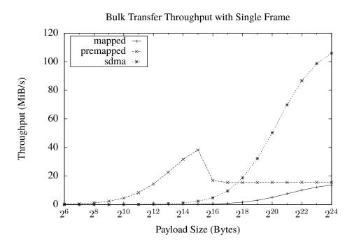
Figure 17: Throughput of bulk transfers using different payload sizes. The same memory region was used in all requests in this experiment.
