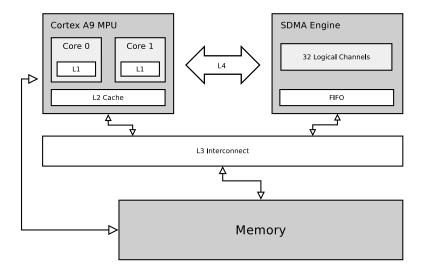
Figure 2: Schematic overview of the SDMA module
