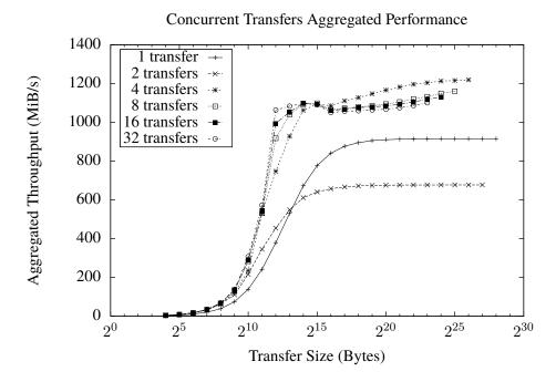
Figure 12: Aggregated throughput when simultaneously running up to 32 burst transfers in parallel.
