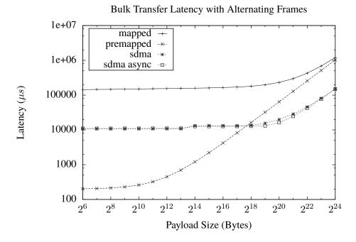
Figure 20: Latency of bulk transfers using different payload sizes with multiple frames used in the requests.
