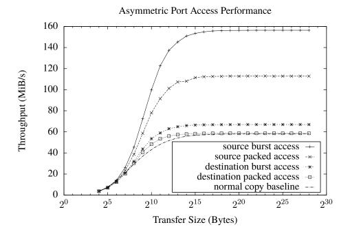
Figure 8: Impact of asymmetric port access on performance. Note that packed or burst access only on the destination port does not show the same improvements as burst/packed access on the source port. The element size was set to 32 bit, burst transfer size was set to 64 bytes.
