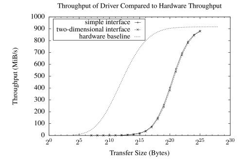
Figure 14: The throughput of the two interfaces compared to the throughput when using the device directly.
