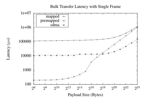
Figure 19: Latency of bulk transfers using different payload sizes with only one frame used for all requests.
